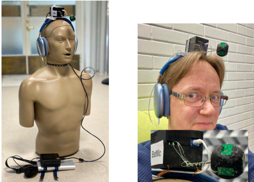
Figure 1. Left: Ultrasonic super-hearing device, where the microphone array and audio interface are mounted to headphones and signal processing is performed in miniature computer inside a black case seen on floor with its power bank. Right: Close-up figures of headphone-mounted parts of the device.
