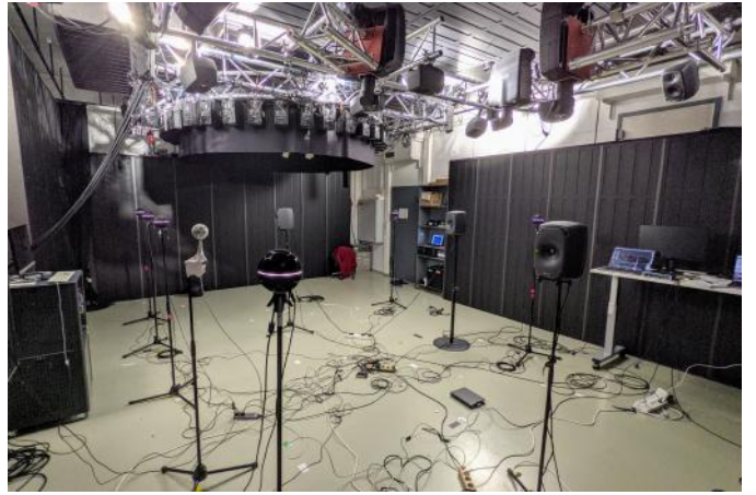
(a) Eigenmike SMA in position R2, 0% absorbers enabled.
