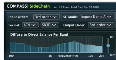
Figure 8: The user interface for the SideChain plug-in, when using the spatial parameters from scene B to process scene A.
