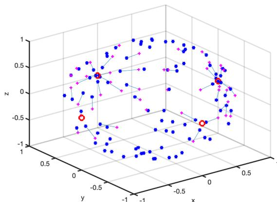
Figure 3: An example of the described direction warping function. The original DoA estimates are depicted as magenta coloured crosses, and as blue asterisks after they have been biased towards the red circle control points ( $\alpha = 1.35$ ).
