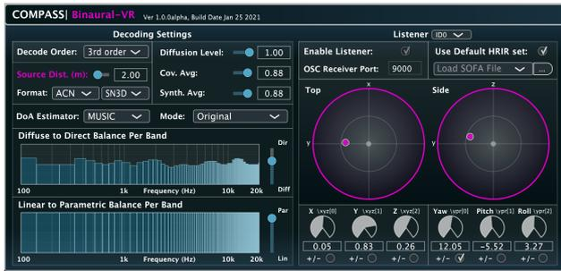
Figure 4: The user interface for the binauralVR plug-in, which supports listener translation around a single receiver and multiple simultaneous listeners.
