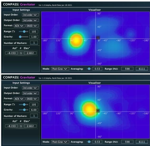
Figure 7: The user interface for the Gravitator plug-in, when  $\alpha = 1$  (top; i.e. not being applied) and when  $\alpha = 6$  (bottom).
