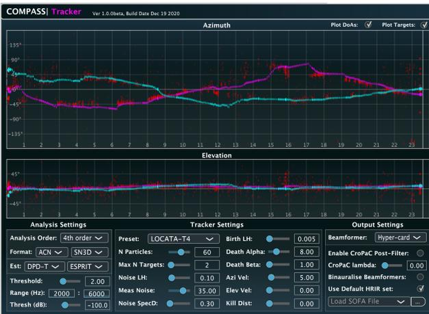
Figure 5: The user interface for the acoustic tracking and beamforming plug-in. The DoA estimates fed to the tracker are depicted in red, and the two target trajectories in magenta and cyan.
