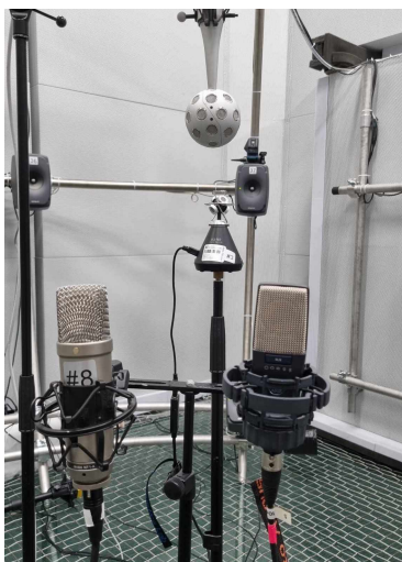
Fig. 2: Arrangement of the microphones and the microphone arrays, which were used for recording the simulated sound scenes, and passing to the different binaural rendering methods under test.
